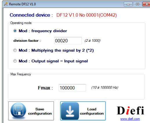
The DF12 is a frequency divider able to decrease frequencies from counter, flow meter or other pulse sources.... It should be used for slow system or limited frequency system to acquire signals. DF12 is fully configured by software. 3 configuration mods are available:
